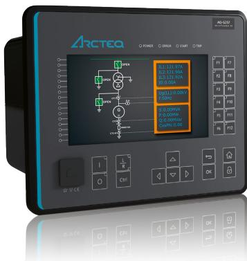
The AQ-G257 generator protection IED is well suited for large machines requiring complete generator protection and differential protection. Up to 9 optional I/O or communication cards are available for extensive monitoring and control applications. Up to 16 RTD signals can be connected for thermal alarming and tripping. The AQ-G257 communicates using various protocols including IEC 61850 substation communication standard.
